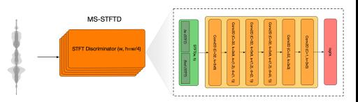
The Multi-Scale Short-Time Fourier Transform Discriminator (MS-STFTD) identifies real and generated audio samples by analyzing spectral and temporal features.
